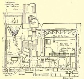
Fig. 280.—Boiler house and generating station of the Remington Arms and Ammunition Company, Bridgeport, Conn.
